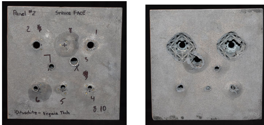
Figure 11. Two SiC reinforcing tiles were pushed completely through an aluminum lattice structure by a 0.50 cal APM2 projectile.
