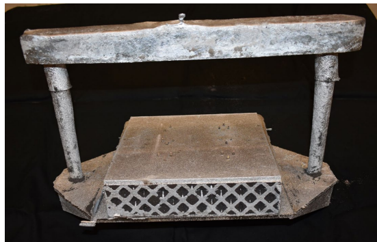
Figure 2. Complete lattice casting with six embedded tiles of varying thickness.
